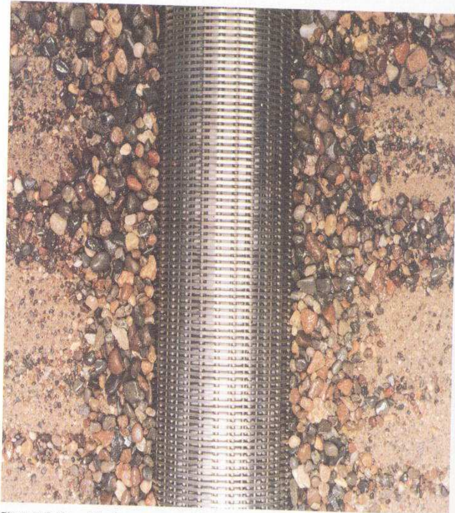
Figure 15.3. Natural development removes most particles near the well screen that are smaller than the slot openings, thereby increasing porosity and hydraulic conductivity in a zone surrounding the screen.
