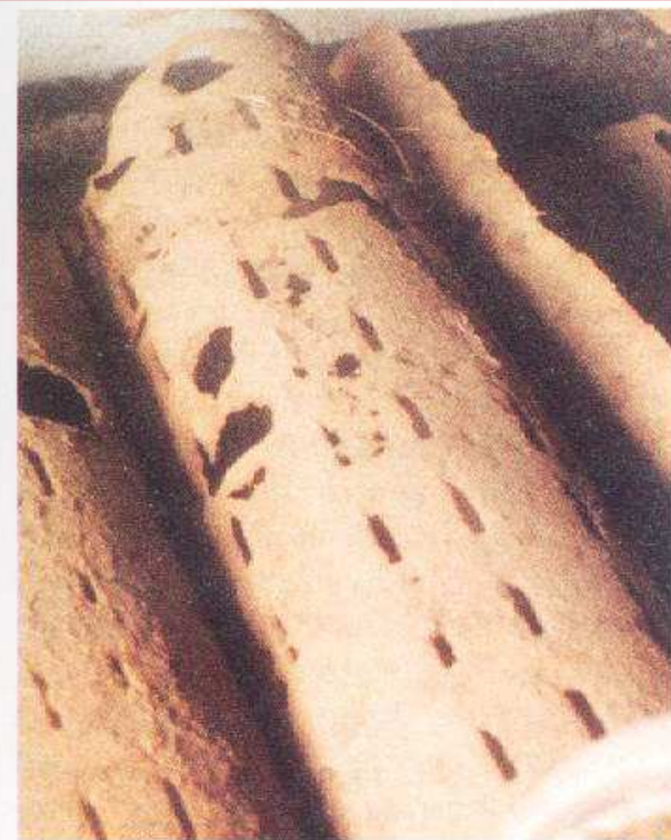
Figure 19.1. Erosion of this well screen resulted from incrustation that caused high flow velocities through the remaining open area.
